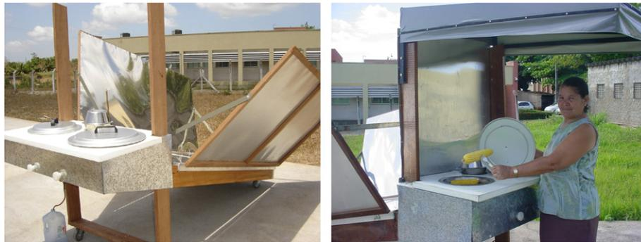
Fig. 3. Photographs of the solar cooker with indirect heating made and tested in Northeast Brazil (1.7 m<sup>2</sup> solar collector, without storage tank, for outdoor use).
