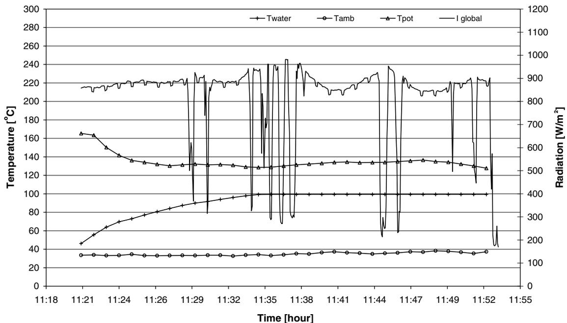
Fig. 4. Hot start field test for a solar cooker with indirect heating, for an average radiation of 837 W/m<sup>2</sup>.
