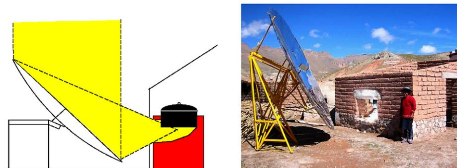
Fig. 2. Fix-focus parabolic collector, a combination of direct and indirect use (type C + D), for an Elementary School in the Altiplano, Argentina.
