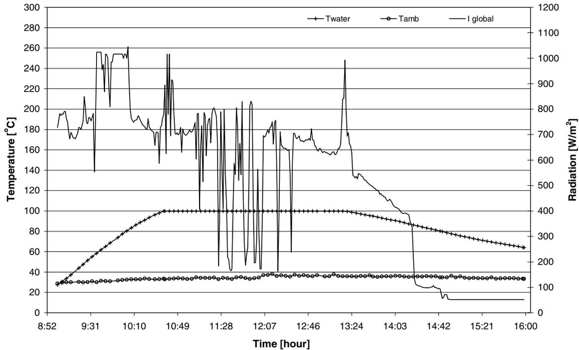
Fig. 5. Field test, with re-orientation of collector, for the solar cooker shown in Fig. 3, for an average radiation of about 700 W/m<sup>2</sup>.
