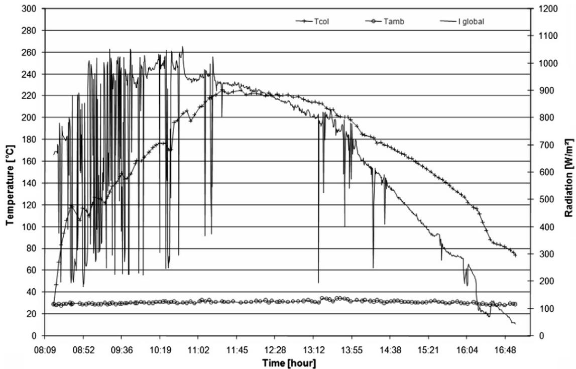
Fig. 7. Stagnation temperature field test (225 °C at 11:30 h) for the solar cooker.
