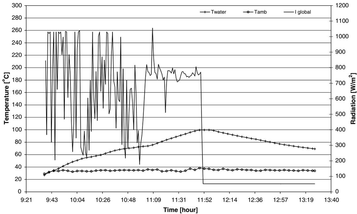
Fig. 6. Heat losses without insolation field test. At 11:50 h, the collector was covered (side reflectors were closed), allowing no radiation to reach the absorber plate.
